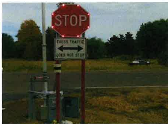
Figure 3-7. Light-emitting Diode STOP Sign
